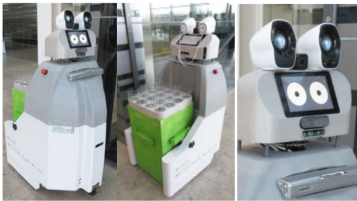
Figure 2. The robot with displayed eyes, the tray with glasses of water on its back, and a goPro camera between the loudspeakers on its head
