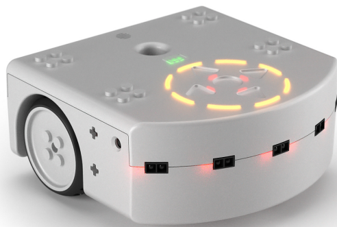
Figure 1. Lateral view of "Thymio," two-wheeled educational mobot (image credit: Mobsya Media Kit, https://media.mobsya.org/ )
