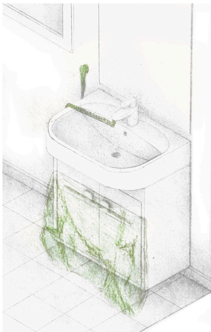
Figure 8: Illustration of the shower head connected to the sink, and a plastic sheet to cover the cupboard, in Sten and Kirsten's ground-floor bathroom, installed by the municipality.
