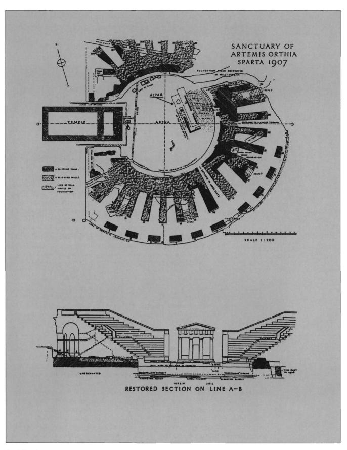
Fig. 6. Plan of the sanctuary of Artemis Ortheia, above, and below, a section also showing the various pavements (Dawkins 1929, Taf. 3f).
