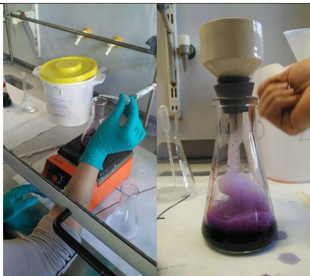
Figure 2: Mixing azo-dye and surfactant and vacuum filtration of the mixture.
