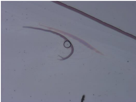
Figure [16]: Optical microscopy test showing these fish-like edges in the mid of our spin casting film. 10x zoom
