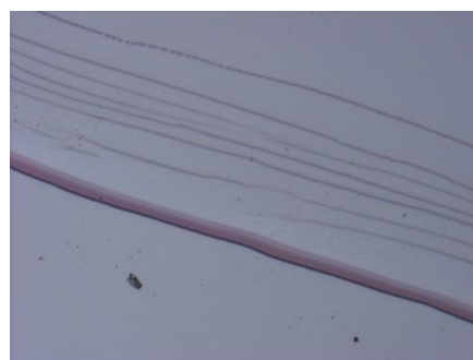
Figure [13]: Optical microscopy test showing an edge in the mid of our spin casting film. 10x zoom
