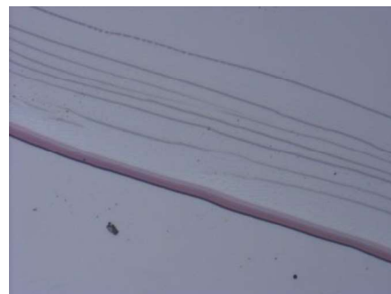
Figure [13]: Optical microscopy test showing an edge in the mid of our spin casting film. 10x zoom
