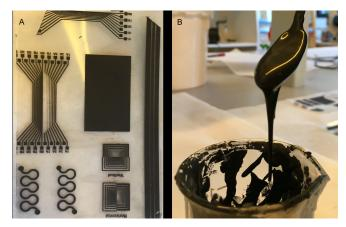
**Fig. 2** In picture a), the synthesized GO-ink is shown. The print is made using the printing setup described in the experimental section. In picture b), the viscosity of the GO-ink used in picture a) is presented. The GO-ink was made using a water-based ink and the synthesized GO. The precise mixture of the ink can be found in the supporting information.
