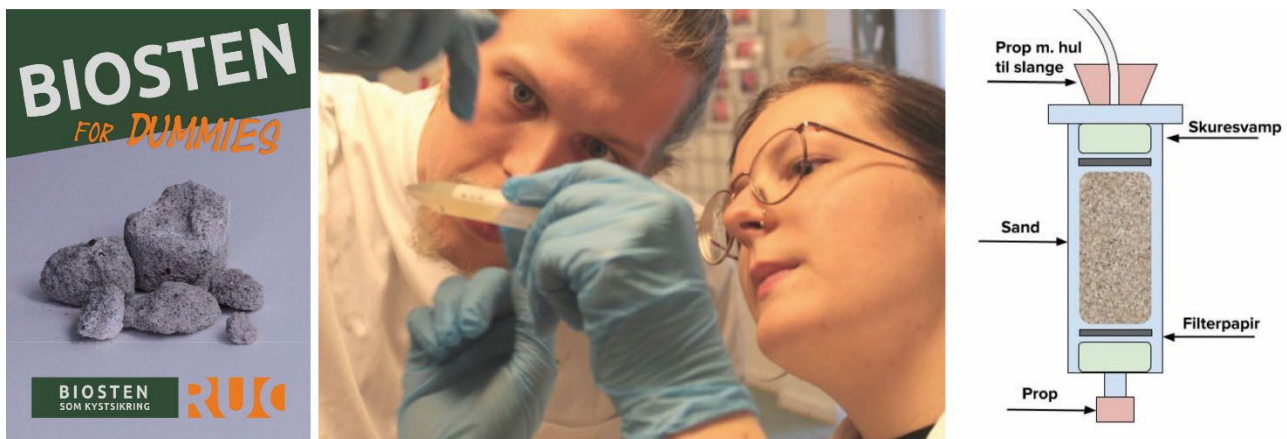
Illustration 1. Biostone as Coastal Protection. a) The group’s short introductory guide to the subject. b) A sample under examination. c) Diagram of the home-designed growth and test chamber.
