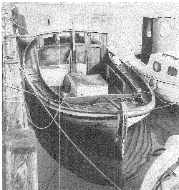
Åledrivrivasen »Rigmor« fra 1912 taget i Svendborg i 1975. Kvasens store bredde, ca. 10 fod, ses tydelig. Endnu ses de oprindelige brede planker i dækket. Foto: forfatteren. Rigmor, an eel drifter, built 1912, photographed at Svendborg in 1975. Its wide beam about 10 feet, can be clearly seen, as well as the original broad planks in the deck. Photo: the author.
