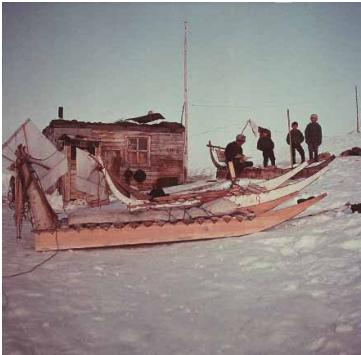
Fig 54. Hunter and district bailiff ( kommunefoged ) Peter Heilmann in front of the family's kit house. He is working on a new shooting sledge, and in the foreground is seen the two types of sledges used. Foremost the Thule-type and rearmost the West Greenland-type. Photo by the author.
