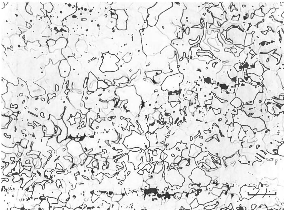
Fig. 67. Polished and etched section through the knife, Fig. 64. Enlarged part of the interior zone of phosphorus rich ferrite with ghost structure. Scale bar 0.07 mm.
