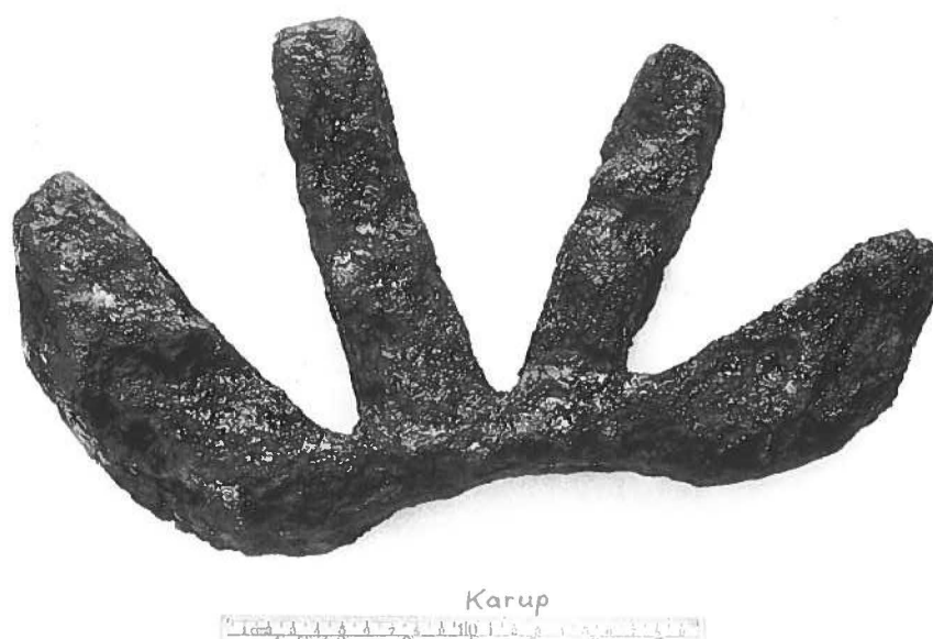
Fig. 2. Typical bloom (Danish, klode ) from Karup, Jutland, Denmark. Weight 8.25 kg. The four parts, when separated, are called klimps . Scale in cm.
