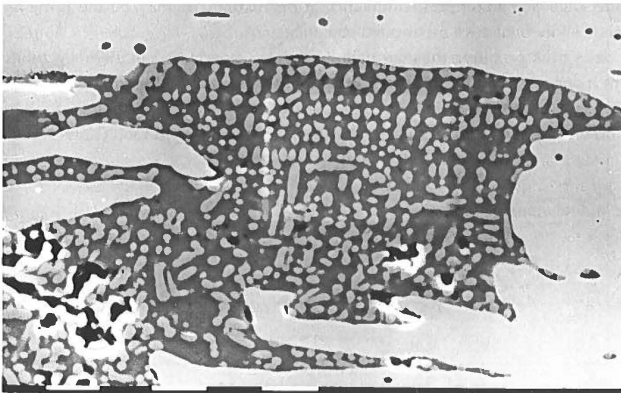
Fig. 72. Another polished section through the nail, no. 18A, Hatherton Bay. The ratio of wüstite to glass varies widely in the same small nail. Some slags are pure wüstite. Puddled iron. Scale bar 0.01 mm.
