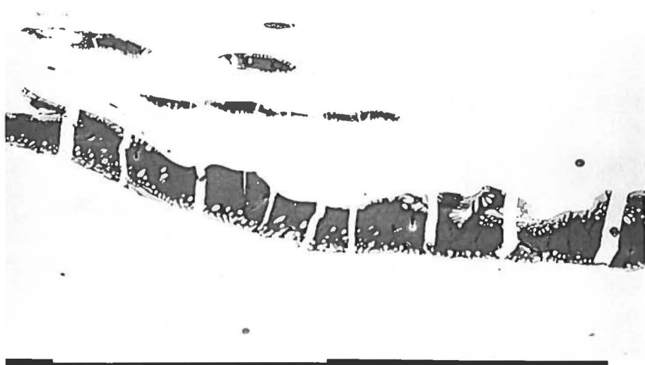
Fig. 46. Polished section through the nail no. 2302 from the Farm beneath the Sand. The slag has been split and displaced during forging. Scale bar 0.1 mm.
