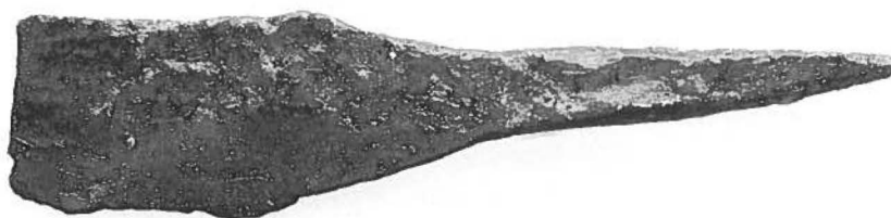
Fig. 45. A knife fragment from Nipaatsoq, no. 618. Although apparently in a good state of preservation, very little metal remained in the sections and also the slags were severely corroded. Length 8 cm.
