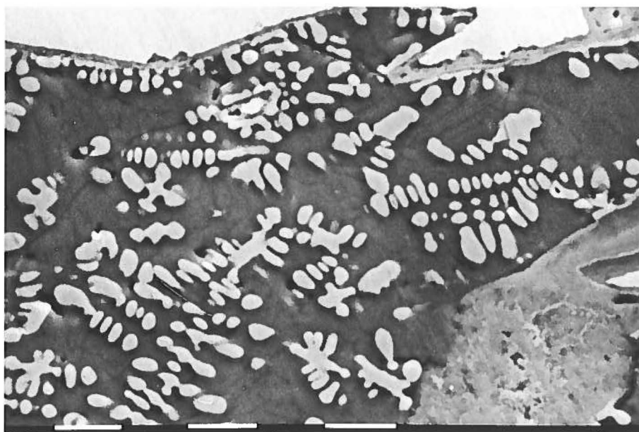
Fig. 35. Enlarged part of the central slag in Fig. 34. Wüstite dendrites in dense fayalite-glass matrix. Above uncorroded iron, to the right akaganeite replacing the iron. Scale bar 0.01 mm.
