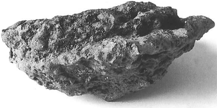
Fig. 3. Purification slag of the plano-convex type (Danish, kalotslagge) seen from the side. Weight 753 g, 15 x 13 cm in cross section and 5 cm high. About 400 AD. Snorup, section 800, Jutland, Denmark. Courtesy Olfert Voss.
