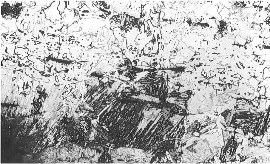
Fig. 66. Polished and etched section through the knife Fig. 64. Martensitic surface zone that merges into phosphorus rich ferrite. Side length 1 mm.
