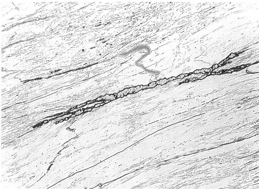
Fig. 57. Enlarged part of Fig. 56. Distorted, sickle shaped taenite band above and a fine line of broken, brittle schreibersite crystals. Matrix is coldworked kamacite. Side length 0.4 mm.
