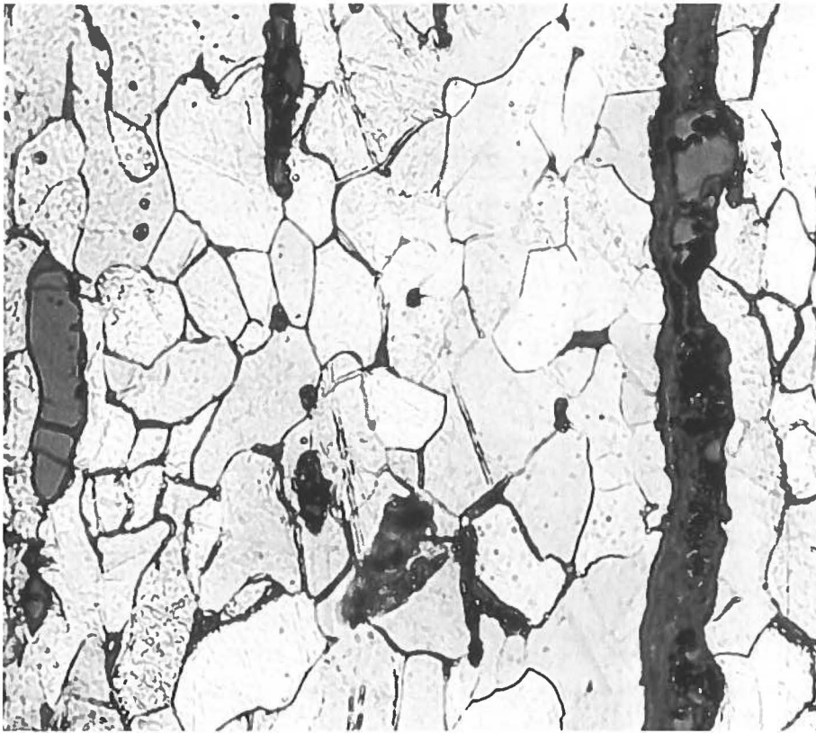
Fig. 61. Polished and etched section through the knife L3.12673, Nuulliit, House 24 B, 1200-1400 AD. Slightly elongated ferrite grains and broken iron-manganese oxide slags with up to 26% MnO. Side length 1 mm.
