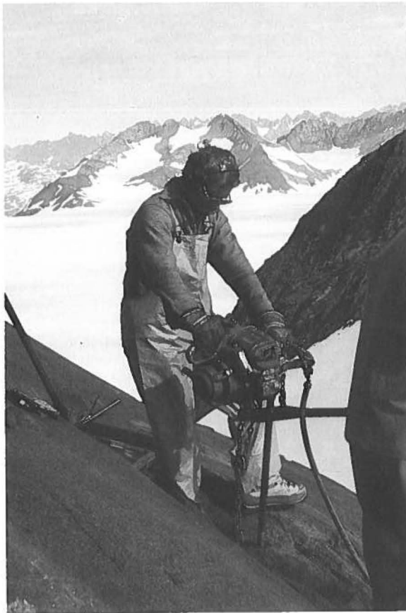
Photo 1. Drilling at Kap Deichmann using hand-held equipment. Lee Barker from RTZ Mining and Exploration Ltd.
