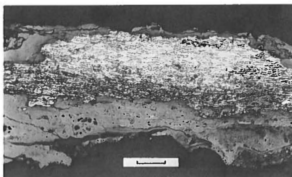
Fig. 55. Cross-section of harpoon blade, L12–814, from Kangâmiut. Elongated, lancet-like ferrite grains. Heavy crust of limonitic corrosion products. Scale bar 200\text{ }\mu\text{m} .
