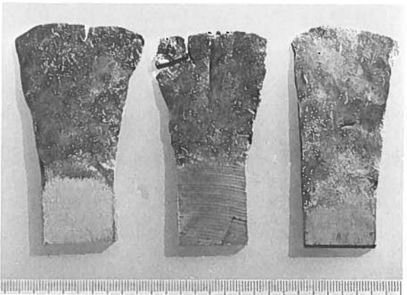
Fig. 26. Three ‘axes’ produced by cold-working steel 42-B (left and right) and a slab of the Cape York iron meteorite (centre). The hammering was continued until fracture occurred. Scale in mm.
