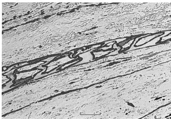
Fig. 14. Cross-section through a meteoritic iron flake. L3-13070 II. Cold worked kamacite and, in the middle, kneaded and microfolded taenite. Scale bar 25 \mu m.
