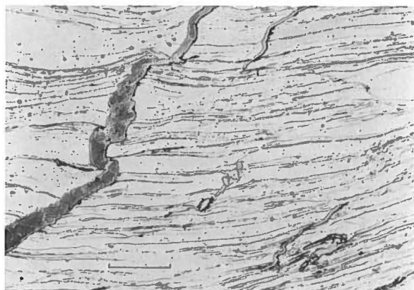
Fig. 15. Cross-section through the meteoritic fragment L3-12631. Distorted kamacite, taenite and rhabdites. Scale bar 100 \mu m.
