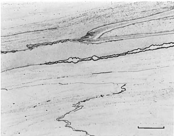
Fig. 24. Section through a shock-deformed meteoritic fragment, L3–12480. Faulted taenite lamellae and irregular, sheared schreibersite crystals. Scale bar 50 µm.
