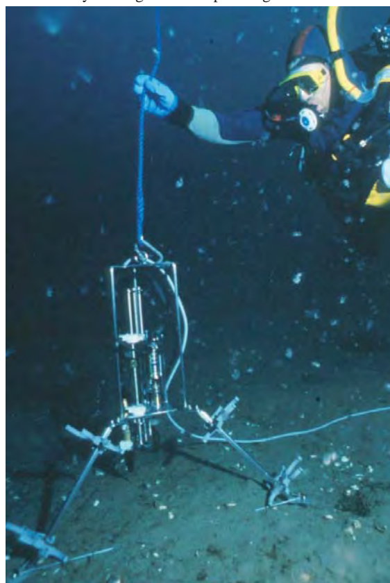
Measuring the microdistribution of oxygen in the upper sediment layer using an in situ profiling instrument.
