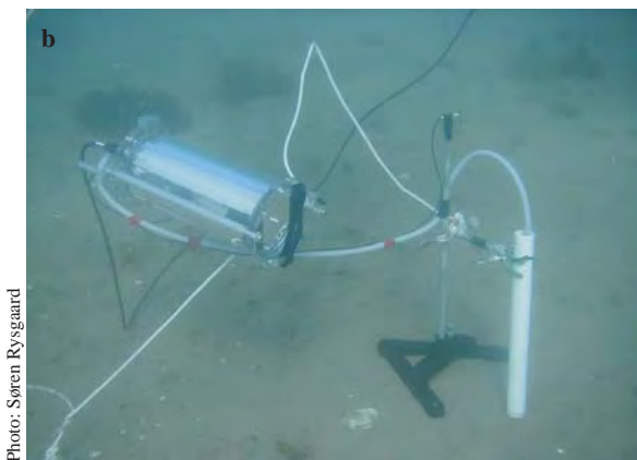
Figure 9.1 Illustration of (a) the oxygen microsensor technique used to measure production of benthic microalgae and crustose coralline algae and (b) of the pulse-amplitude-modulated (PAM) fluorometer.
