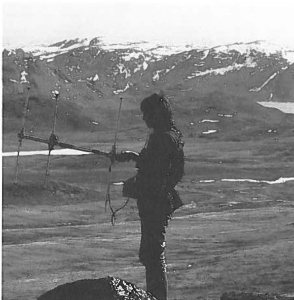
Figure 16. Radio-tracking using a hand held Yagi aerial and portable radio receiver with headphones. Background shows part of study area in mid-June, following main thaw.
