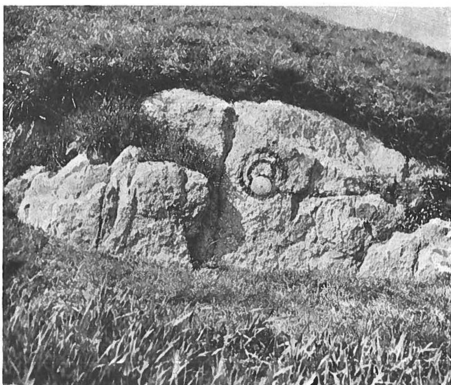
Fig. 11. Levelling-point II in the Colony-Manager's garden at Julianehaab. Round the main bolt are painted two concentric rings.
