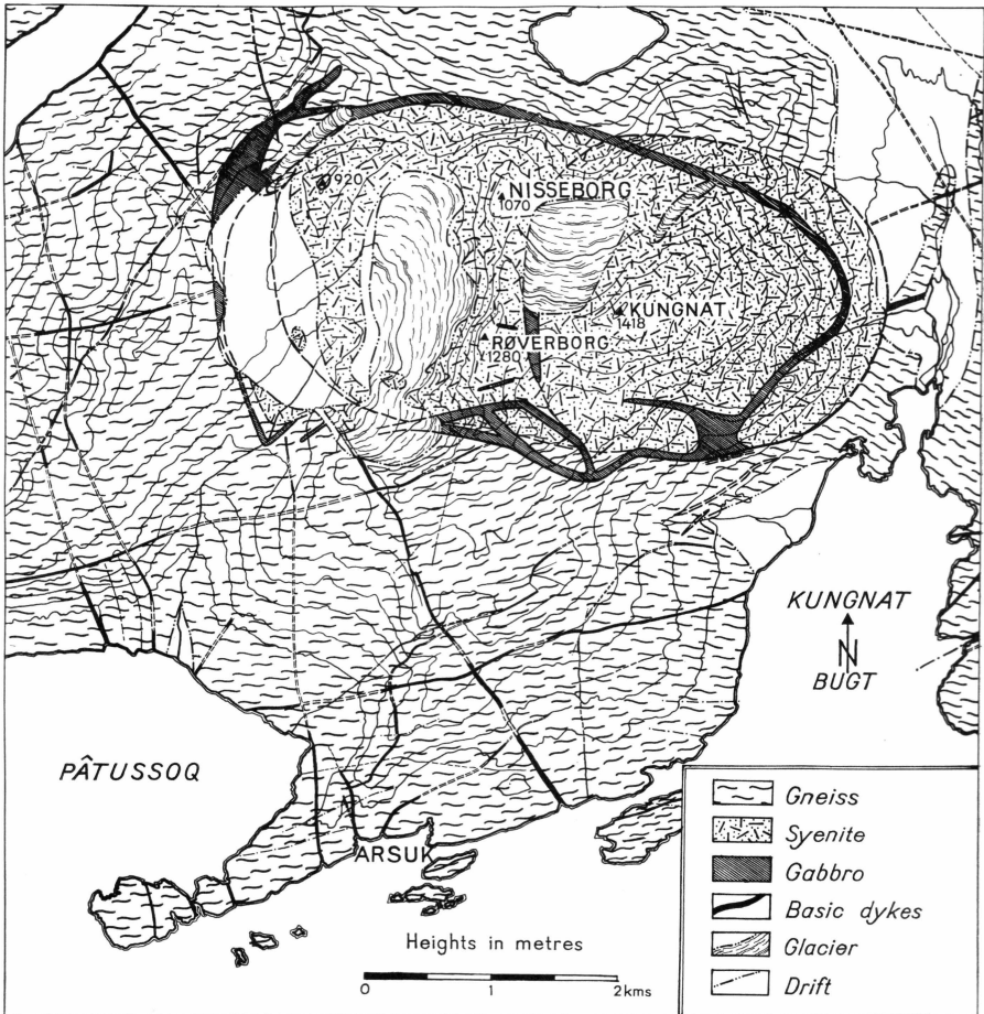
Fig. 3. Map of the Kungnât complex indicating the extent of drift and permanent ice, and showing the main dykes in the region.
