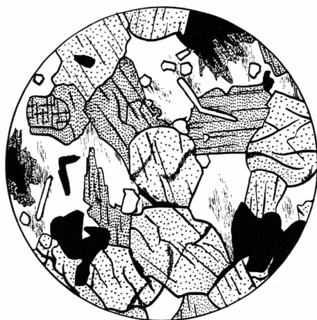
Fig. 36. Primary precipitate fayalite and pyroxene, slightly modified by interprecipitate growth, in the basal part of a rhythmic unit from the lower banded group. These are accompanied by feldspar, apatite, biotite and anhedral ilmenomagnetite. Uncrossed nicols. \times 20 .
