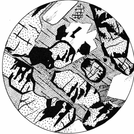
Fig. 37. Fayalite crystals in a syenite from the western upper layered series, partly pseudomorphed by ore and poikilitically enclosed by hornblende. Uncrossed nicols \times 20 .
