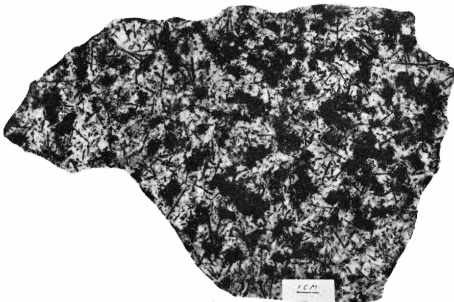
Fig. 9. Gabbro with long bladed pyroxenes. Cross-sections exhibit igneous lamination. Dark areas are serpentinised olivine.
