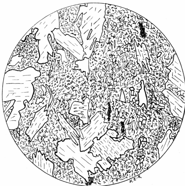
Fig. 15. Greenstone or green amphibolite. Short-prismatic uraltic hornblende individuals in a fine-grained groundmass. The three small ellipsoidal grains bottom left are olivine. North-south in the fourth quadrant are a number of scapolite grains. (G. G. U. 36054. Ab. 9 \times magn. lin.).
