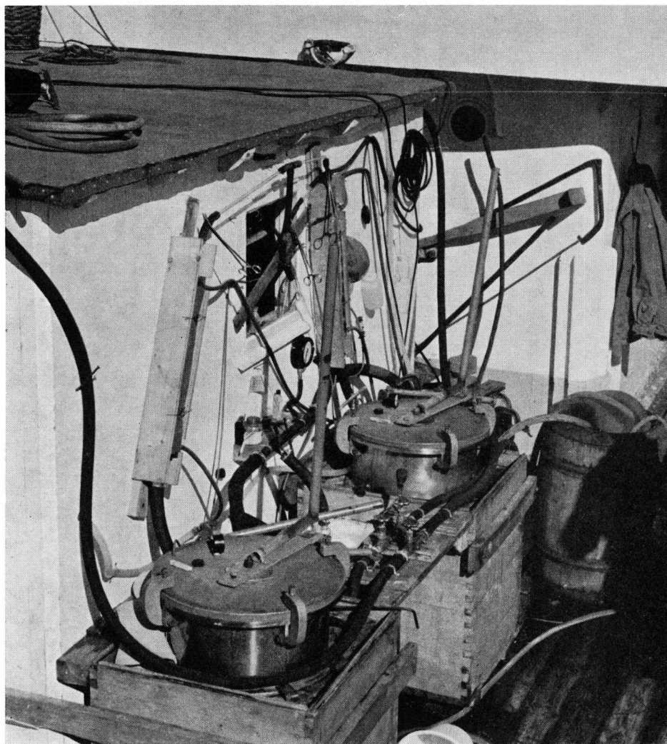
Fig. 3. Vacuum boilers with reflux condensers outside deck laboratory. CO 2 absorber located inside laboratory could be observed through window.
