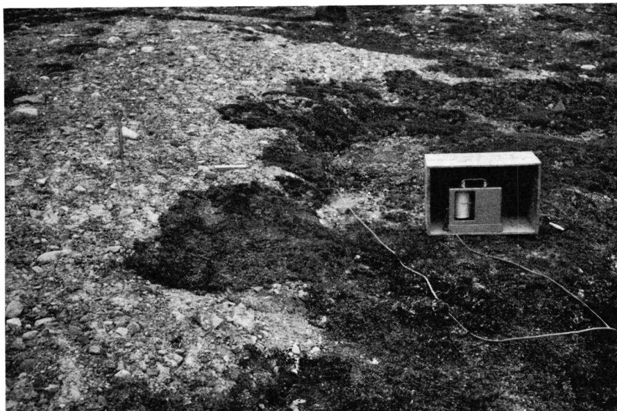
Fig. 23. Experimental site 8. Thermograph 8A installation. View upslope. 16-cm rule marks location of bulb. (2 Aug. 1958.)
