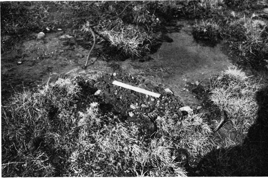
Fig. 27. Experimental site 8. Thermograph 8D and 8E installations. Bulb 8D at depth 5 cm; location and orientation indicated by 17-cm rule. Bulb 8E flush with surface at left of bulb 8D and at right angles to it. View upslope. (3 June 1960.)
