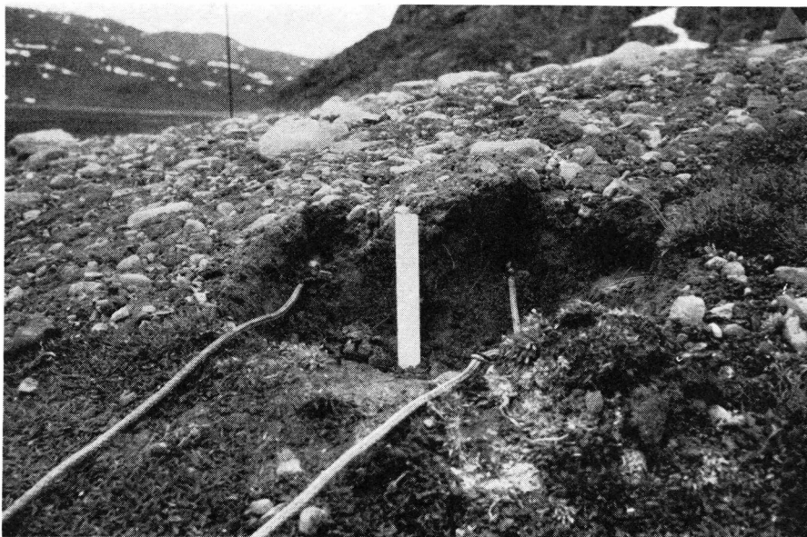
Fig. 24. Experimental site 8. Thermograph 8B installation. View west prior to backfilling. Bulb 8B1 at right, bulb 8B2 at left. 17-cm rule as scale. (21 Aug. 1960.)
