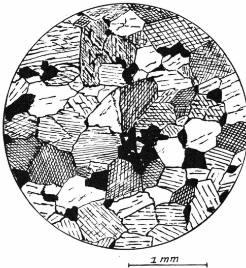
Fig. 15. Hornblendite, Kuánit area. The rock shows an equigranular, idioblastic texture. The ore grains are interstitial between the hornblende crystals. (46823).
