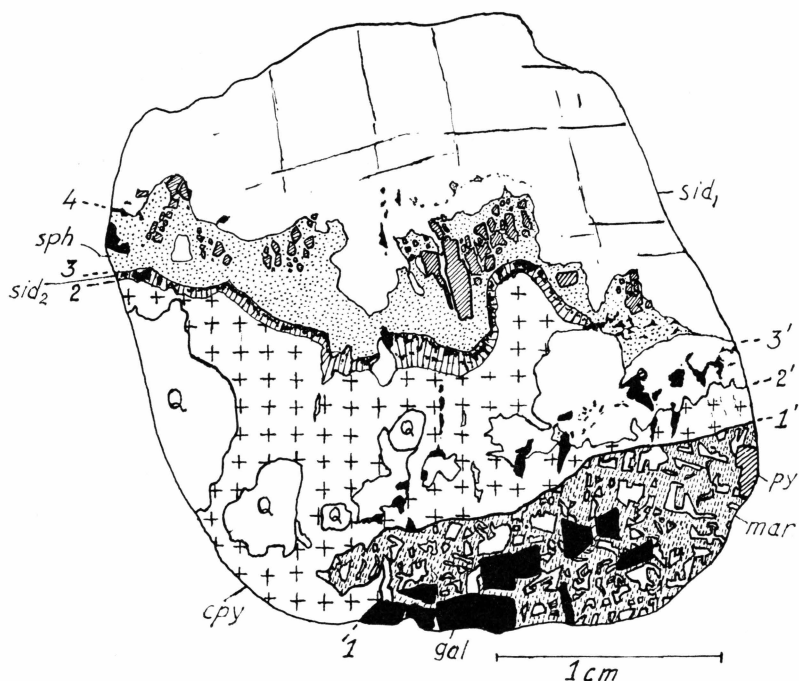
Fig. 2. Polished section 821; sid_1 – coarse-grained siderite of the envelope of the nodules, sid_2 – fine-grained recrystallized siderite of the mantle of the nodules, py-pyrite, gal-galena, sph-sphalerite, cpy-chalcopyrite, mar-marcasite, and Q-gangue. The section shows a part of a nodule with several zones as described in the text of the paper. From bottom to top of the figure the following zones can be recognized: (a) A part of the core of the nodule with its outer boundary 1–1'; the core is filled with a finely developed, cavernous marcasite dendrite showing a rectangular pattern of the dendritic sheets; inclusions of euhedral galena and pyrite in the core of the nodule have apparently crystallized as cavity fillings; (b) The chalcopyrite zone with its outer boundary 2–2'; the inclusions of siderite and galena in this zone are apparently replacement relicts; (c) A thin zone of fine-grained recrystallized, columnar siderite between 2 and 3; at the external side of this zone a very thin band of galena borders directly to the sphalerite zone, note that this galena band is concordant to the boundary of the sphalerite zone; for details in this zone see text-figures 11 and 12, plate II fig. 2 and plate III figs. 1 and 2; (d) The sphalerite zone between 3–3' and 4; this zone contains inclusions of siderite and pyrite; note the scalloped inner boundary of the sphalerite zone with convex bulgings towards the core.
