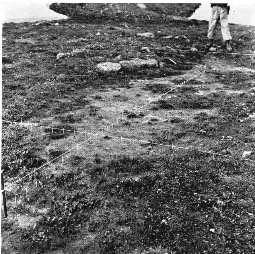
Fig. 50. Experimental site 15, showing lines of target dowels on the small gelifluction lobe. Photo 28 July, 1957.
