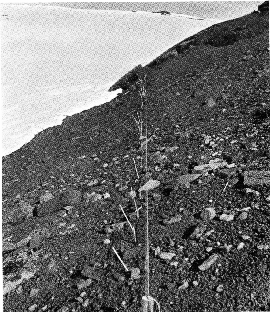
Fig. 61. View along target line of ES 16, showing movement of dowels from 17 Aug., 1957, to 31 May, 1960. From WASHBURN, 1967, Fig. 37.
