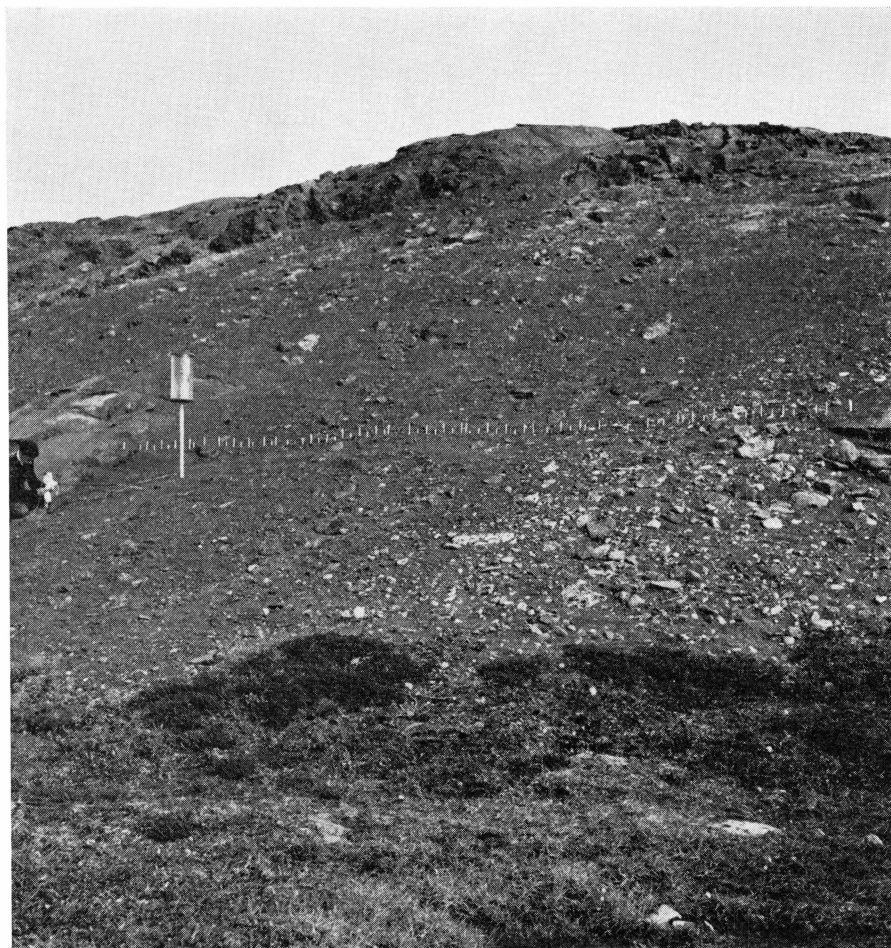
Fig. 58. Experimental site 16. View northeast, diagonally upslope. Target line extends between trap outcrops in middle ground; mass-wastingmeter 16 is below target line at left; 22 Aug., 1957. From WASHBURN, 1967, Fig. 33.
