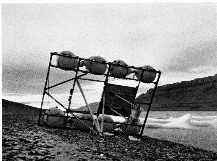
Fig. 18. The raft.—Plywood deck plates removed to show construction.
