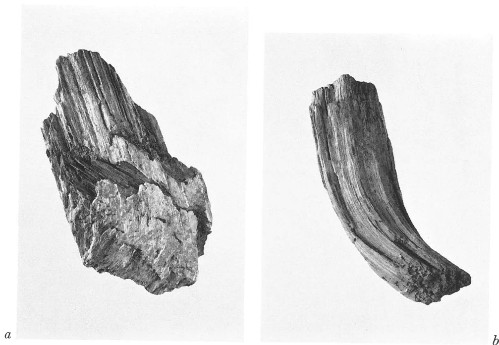
Fig. 1. a) Fibrous xonotlite sample with the fibres arranged in groups. The fibres within each group are oriented parallel to each other but are not parallel from group to group. b) Xonotlite specimen with strongly bowed fibres, arranged in stalks, which result in a distinctly ribbed surface appearance.
