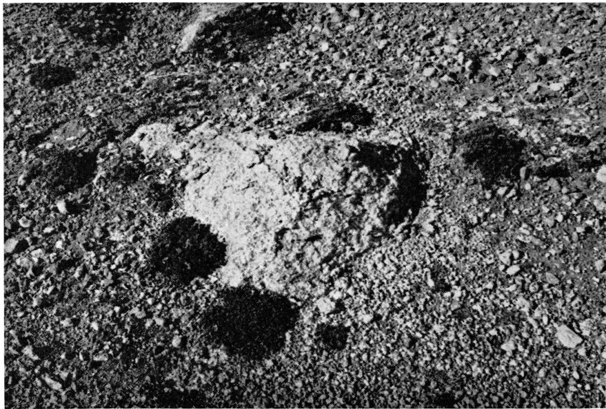
Fig. 25. Deep-seated weathering of a crystalline boulder. The rock matrix can be easily crushed by hand.
