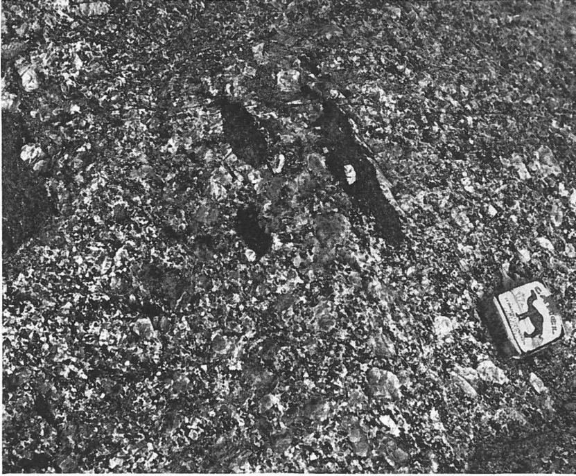
Fig. 5. Big-feldspar granite (variety B<sub>2</sub>, symbol g).
