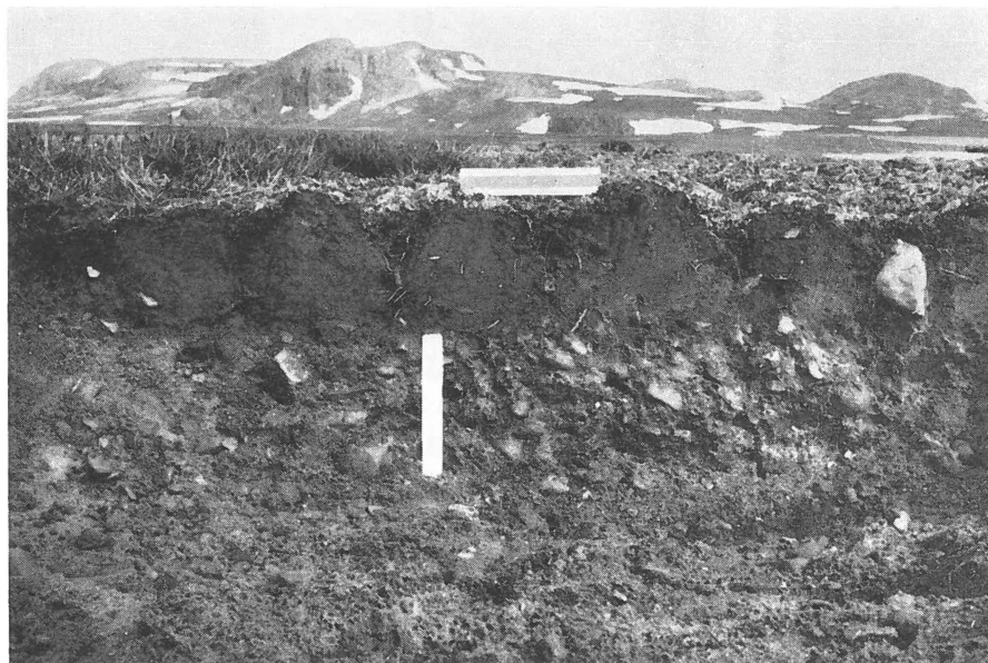
Fig. 21. Soil profile on 25-m emerged delta remnant, showing small sorted polygons (excavation 60-7-23). Scales are 17-cm rules. 23 July, 1960 (from WASHBURN, 1969, Fig. 100).
