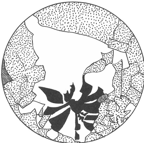
Fig. 17. Spherulitic structure in microgranite. Stipple = alkali feldspar. Solid black = radiating feldspar structure. The feldspars making up this structure are not optically continuous, but the quartz (unornamented) between them, is in optical continuity. Irregular cross-hatching = biotite. High power, diameter of field = 0.5 mm. Specimen 948. See also Plate 1, fig. 2.
