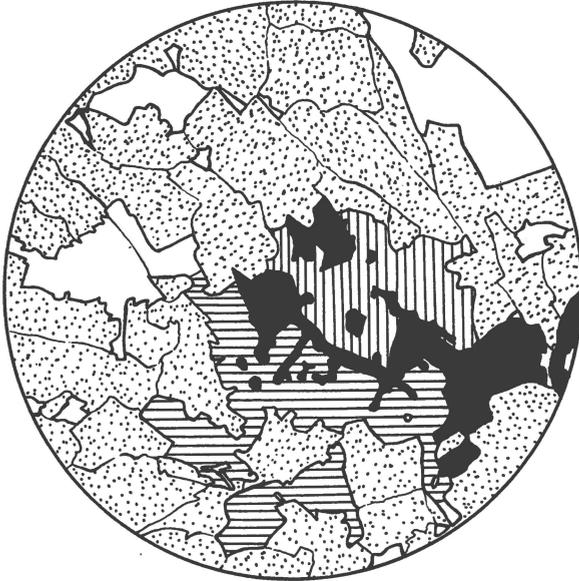
Fig. 12. Textural relationships between quartz and feldspar in a soda granite (945). No ornamentation = quartz; cross-hatching = optically continuous patches of quartz; stipple = feldspar; solid black = single continuous feldspar.
