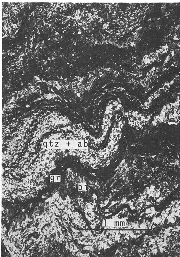
Fig. 6. Graphite-rich semipelite, see p. 26, (ab) albite, (bi) biotite, (gr) graphite, (qtz) quartz. Plane polarised light (GGU 164450).
