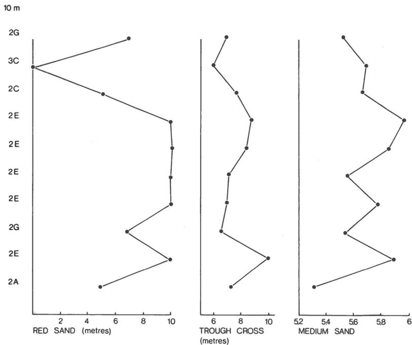
Fig. 66. Succession logged at K504 in Scott Bjerg red sandstone member. Classification of 10 m samples is shown with proportions of red sandstone, cross-bedding and medium-grained sandstone.
