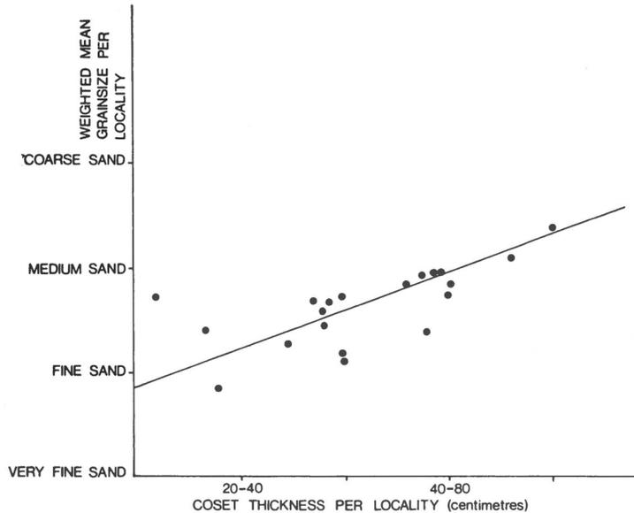
Fig. 49. Diagram showing relationship of mean grain-size per western sequence locality (weighted for thickness), and mean coset (same-structure) thickness for cross-bedding.
