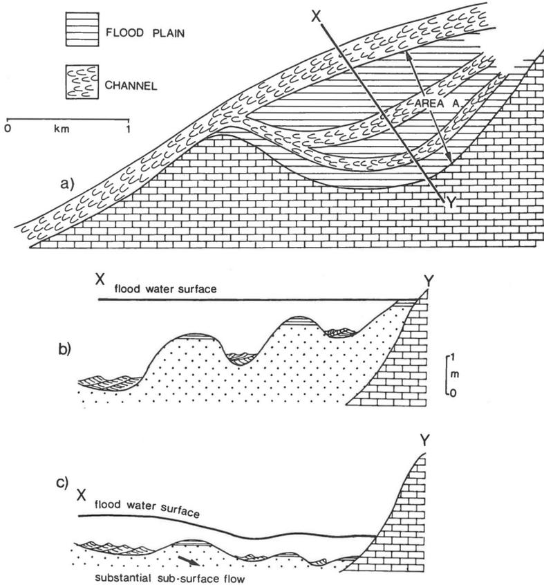
Fig. 69. Sketch map (a) and sections (b and c) illustrating possible situations on fan margins. Pre-Devonian limestone basement is shown by a brick symbol. Sections b and c illustrate two alternatives, in the second of which substantial water flow percolated into the alluvium.
