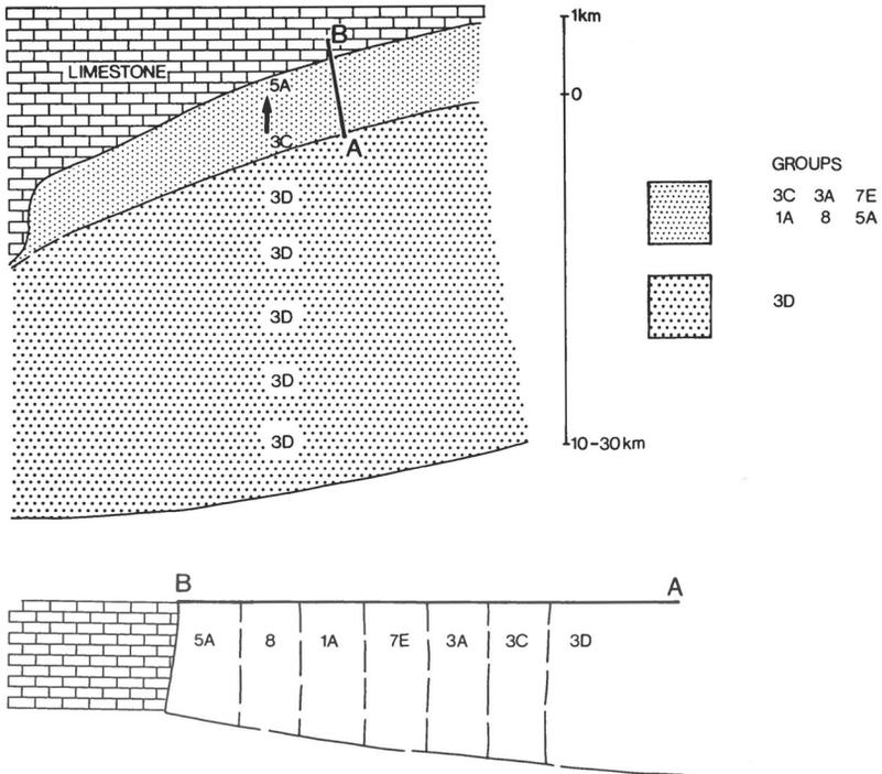
Fig. 68. Sketch map and vertical plane section illustrating sample group relationships generalised for the margin of an alluvial fan. The characteristically marginal sample groups are typically developed in an embayment of the basement of pre-Devonian limestones.
