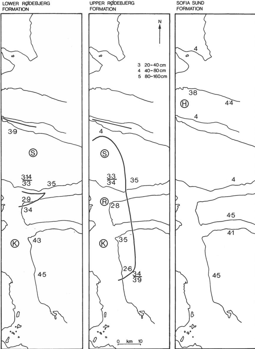
Fig. 46. Maps showing mean coset (same structure) thickness for cross-bedding for localities in the three stratigraphic units of the western sequence. Numbers are thicknesses expressed on an arbitrary scale in which thicknesses of 20–40 cm were scaled as 3, 40–80 cm were scaled as 4, 80–160 cm were scaled as 5. Other conventions described in caption of Fig. 45.
