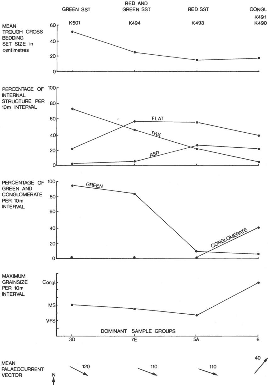
Fig. 55. Diagram to illustrate change of certain properties on Scott Bjerg, in lateral transition from sample group 3D to 7E, to 5A and to 6. Properties plotted are cross-bedding set thickness, percentage of various internal structures, percentage of green sediment and of conglomerate, maximum grain-size and palaeocurrent.
