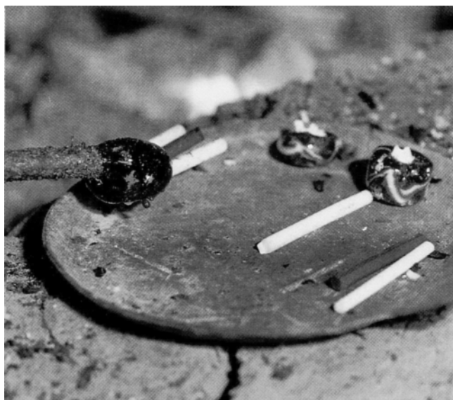
Fig. 6. Two white and a red thread being joined on blue glass as a thread band. In the pan are two further white and a red thread, and two finished beads being annealed. Photo S. Heinesen, HAF.
