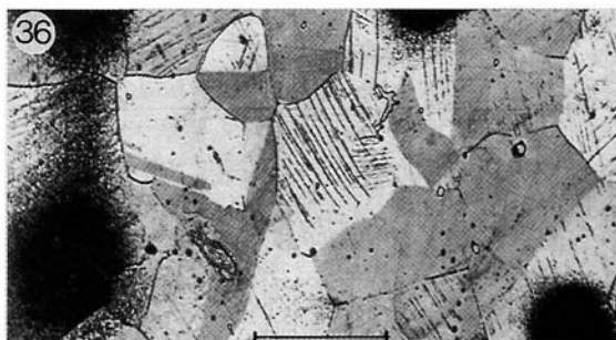
Figs. 29–36. Fig. 29. No. 3. B 1094. Low-flanged axe, 190 g. Fig. 30. Vickers (5 kg) and Microvickers (100 g) hardness of sections A and B. Fig. 31. Segregated and worked structure at A with microcrack (above right). Scale bar 0.5 mm. Fig. 32. Cored and recrystallized grains in the interior of B. Scale bar 0.1 mm. Fig. 33. No. 4. 11073. Low-flanged axe. 480 g. Fig. 34. Vickers (5 kg) and Microvickers (100 g) hardness of sections A and B. Fig. 35. Cored and recrystallized grains in the interior of B. Scale bar 0.5 mm. Fig. 36. Recrystallized and cold-worked material in flanges of B. Scale bar 0.2 mm.
