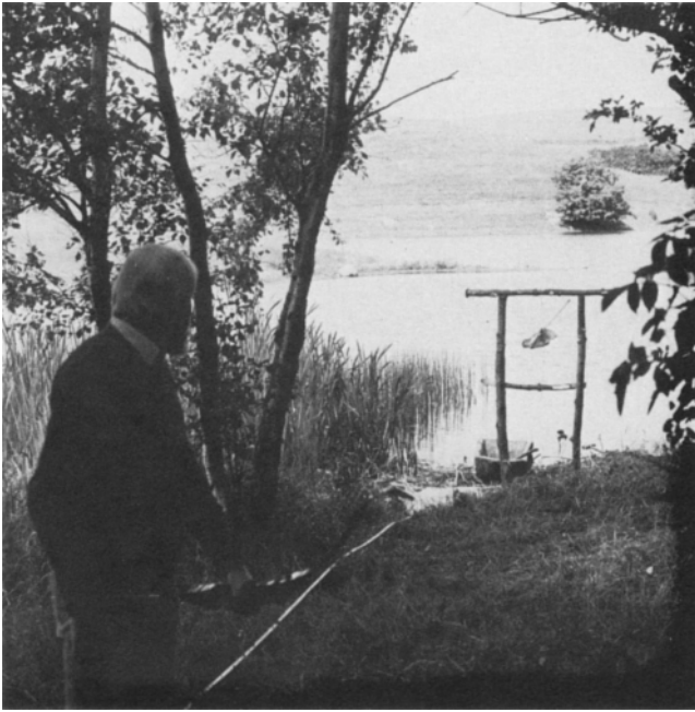
Fig. 1. Snapshot of the shooting experiments. An arrow has just been fired against a shoulder of pork suspended in a wooden frame. The lake in the background ensured that arrows missing the target remained undamaged.
