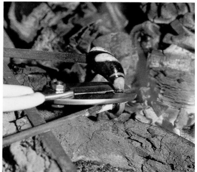
Fig. 13. Reticella thread being cut away with the scissors. Photo S. Heinesen, HAF.
