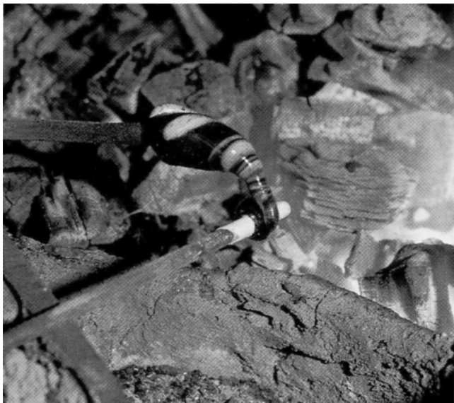
Fig. 12. Reticella thread being wound on to a blue bead. Photo S. Heinesen, HAF.
