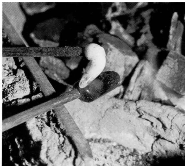
Fig. 9. White threads being melted directly on to an end of blue glass for reticella beads. Photo S. Heinesen, HAF.
