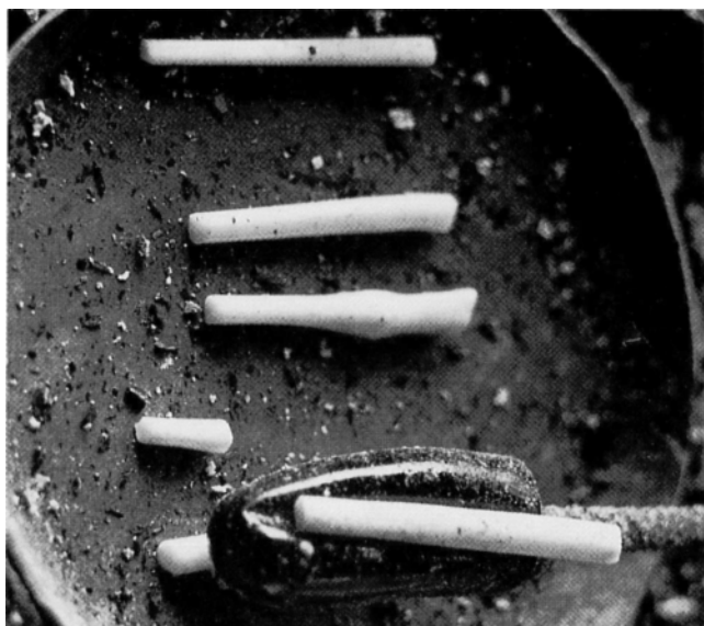
Fig. 8. White threads being rolled on to an end of blue glass. Photo H.S. Rasmussen, HAF.
