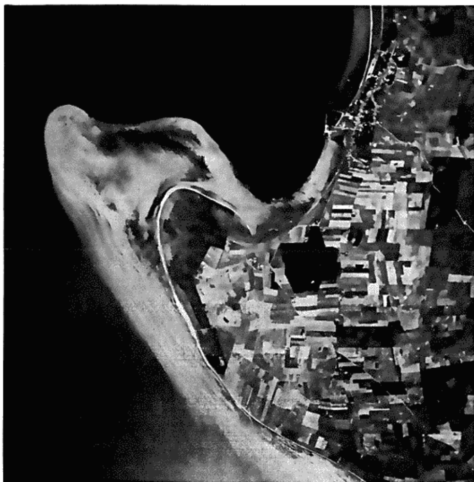
Fig. 7. Ahl Hage , a cuspate foreland at the entrance to the bay of Æbeltoft Vig (cfr. fig. 2, II). The foreland has developed on a wide platform of sand, Sandhagen, built up by beach drifting into the bay. The whole foreland complex acts as a breakwater for the harbour of Æbeltoft constructed in the bay behind it. The grain size of the beach material is diminishing from south to north. The dark shade in the interior of the foreland indicates the conifer plantation established to protect the agricultural area against blown sand.
