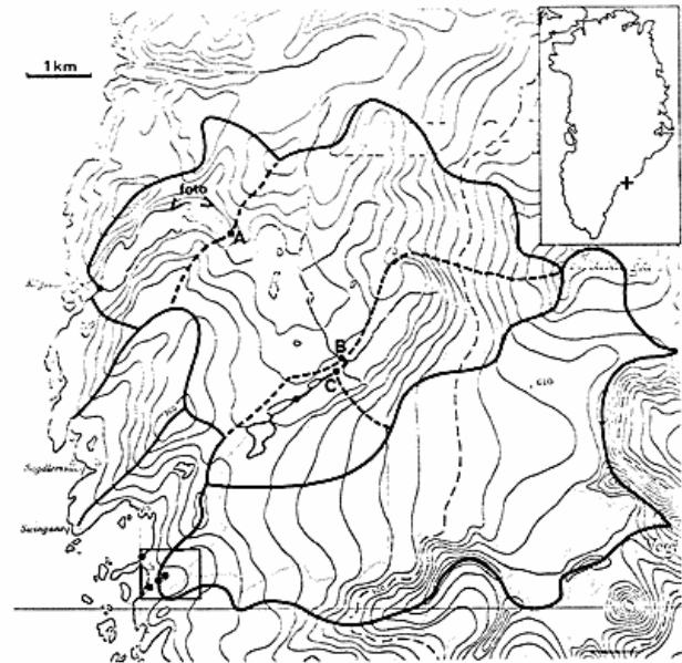
Fig. 1. Survey map. Lines indicate watersheds, dots indicate measuring stations. The area within the frame is shown in fig. 2.
