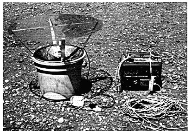
fig 13: The light traps used: a. A portable Heath trap with MC battery. b. A modified Robinson trap with Honda E-300 generator. Notice the Plexiglass coverplate.
