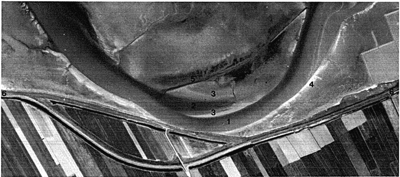
Fig. 3. Aerial photo from 1973 of part of the Juvre Priel. 1. ebb channel. 2. flood channel. 3. flood bar. 4. levees. 5. tidal creek. 6-6. Juvre Dike. Approximate scale 1:12 500.
