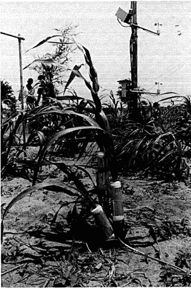
Fig. 2. Photo of Sapflow-gauges installed on millet.
