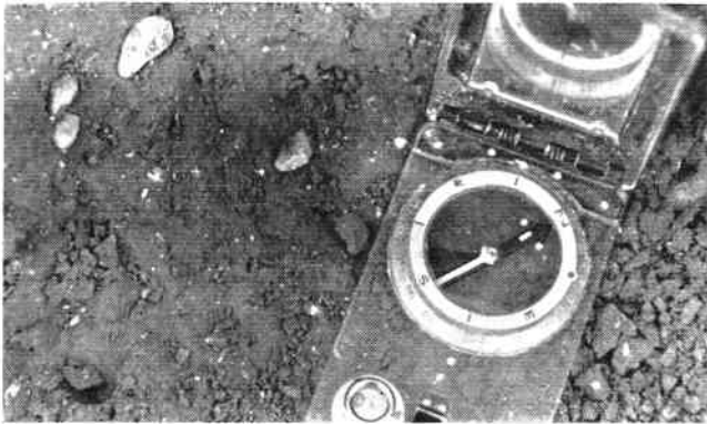
Fig. 3. Snapshot from analysis No. 9. The compass indicates the orientation of till pebbles "in situ". Juni 1970.
