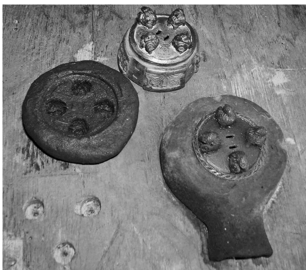
Figure 13. Mould B. 'Smis' replica-brooch tried as aid for separate top for upper-mould. Result partly negative.
