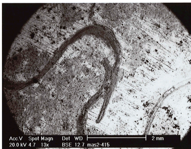
Figure 3. The 2 mm overlap between two copper wires in the razor from Arnitlund (Photo: A. Jouttijärvi).
