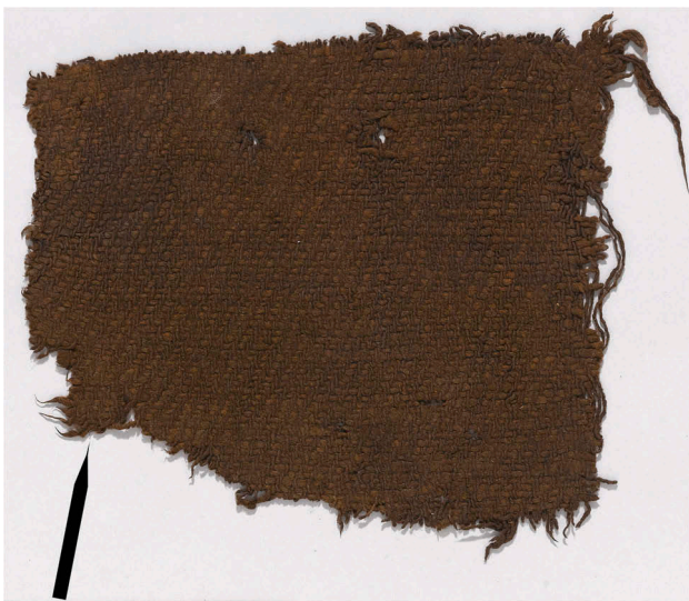
Figure 2. Sampling from textile fragments. Sampling is most often done near open edges or holes where degradation can be more advanced.
