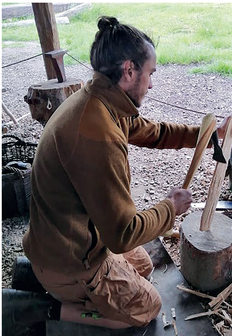
Figure 3. Wood for the blades was produced from radially split blanks that were shaped using an adze to a precise length, with, and thickness (Photo: H. Lyngstrøm).
