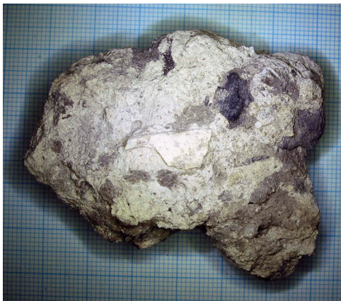
Figure 3. Lump of lime from kiln FG-A118 with charcoal and bone fragments. Photo: P.S. Henriksen.
