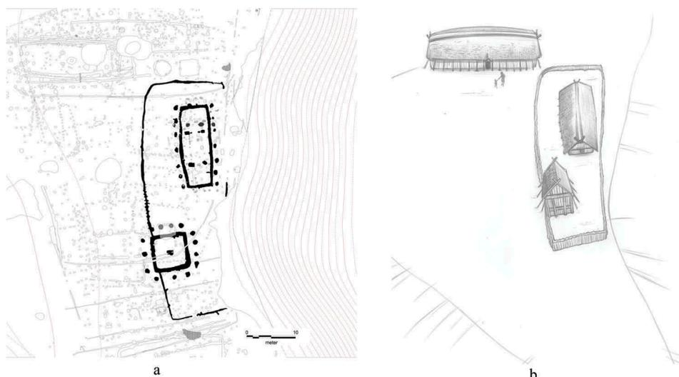
**Figure 5.** (a,b). Combining one of the northern halls with the fenced area, the north–south-oriented house (K2) and the tower (K1) provide a sort of possible minimum settlement overview in the first half of the eighth century. The lighter areas in the northern wall and two posts of the tower were found underneath a pit-house, which bear witness to the depth of the supporting parts of the structure. To the left is a reconstruction of that particular phase. Drawing: Tom Lock.
