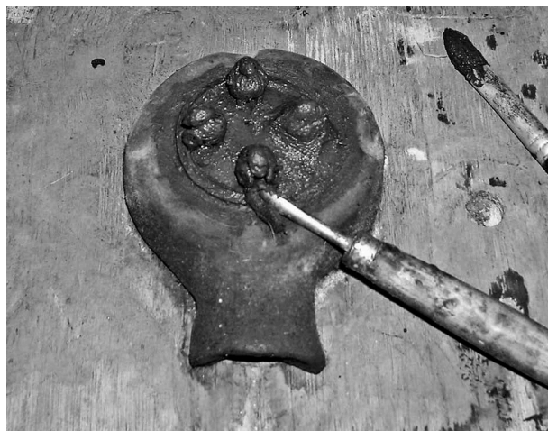
Figure 14. Mould B. Adding slurry and impression loam with spatula and brush to knotty animals on wax model.
