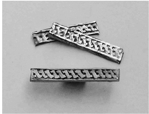
Figure 22. Positive die with steep rope-cord ornamentation for producing silver plating. Replica.
