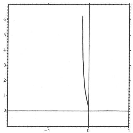
Fig. 3.2. The region of contractivity in the (0.5,2)-norm of the fixed-step second-order BDF.
