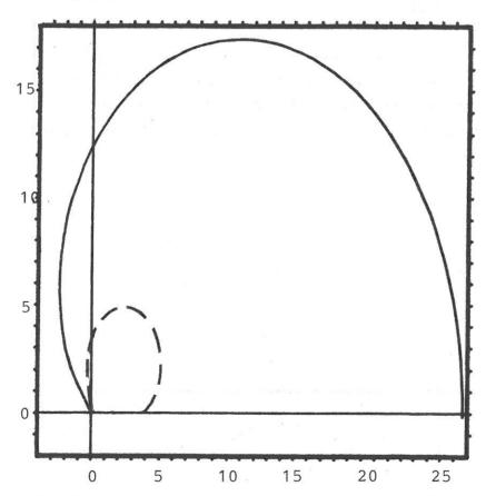
Fig. 5.2. The region of absolute stability (dashed line) and the region of contractivity in the (0.2,4)-norm of the third-order 3-step one-leg formula with  $\Theta=\sqrt{5.53}-1.5$ , B= 0.6.
