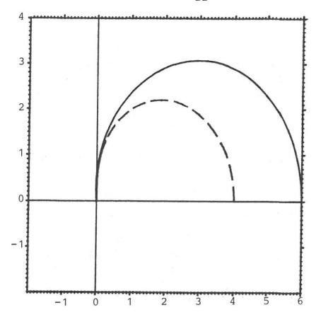
Fig. 3.1. The region of absolute stability and the region of contractivity in the (1/3,2)-norm of the fixed-step second-order BDF.
