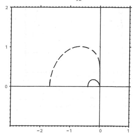
Fig. 5.3. The region of absolute stability (dashed line) and the region of contractivity in the (0.2,4)-norm of the fourth-order 4-step one-leg formula with  $\Theta=B=0.6$ .
