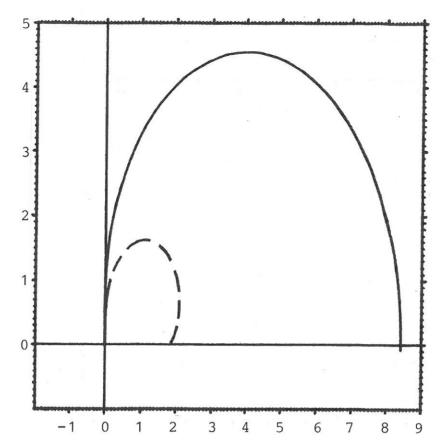
Fig. 5.1. The region of absolute stability (dashed line) and the region of contractivity in the (0.2,4)-norm of the second-order 2-step one-leg formula with  $\theta$ =0.54, B=0.6.
