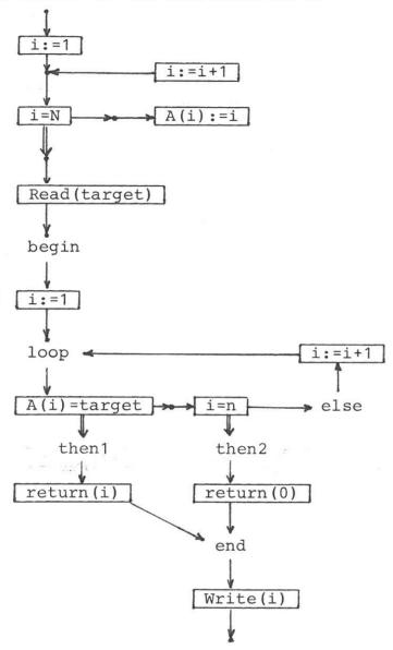
One of the disadvantages of flowcharts is they become very bulky, but converting flowcharts to graphs by labelling all arrows and dropping frames gives more concise models. For us a graph consists of labelled vertices and labelled directed edges; in a graph model of a program the vertices correspond to control points and the edges correspond to program statements.
