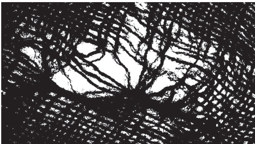
Fig. 4. Fig. 3 after a threshold. All pixels having a value below zero are coloured black and all pixels having a value above zero are coloured white. By simply counting the white pixels and comparing this number with the total number of pixels in the image one can get a percentage of how much background is visible through the fabric (Photo: authors).
